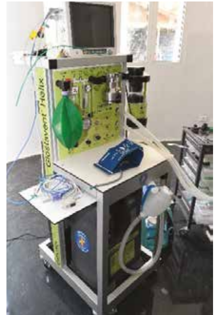
Figure 20. An open circuit anaesthetic machine designed for the LMIC environment.
