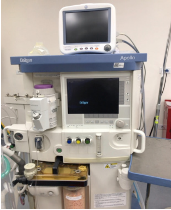
*11ET, #064 Benchmark compliant closed circuit anaesthetic machine that was purchased new.
