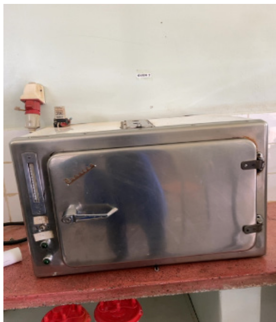
03UG, #005. Acceptable, used within the past 7 days, no safety concerns, satisfactory performance. However, the device does not reach designated temperature and pressure.
