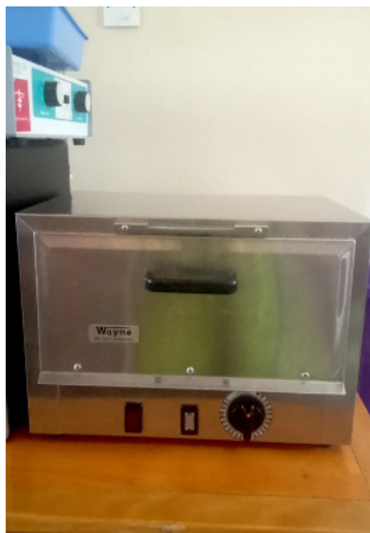
23MW, #012 The only benchmark compliant autoclave at this facility is a dry heat steriliser.
