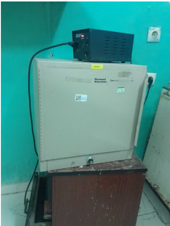
04ET, #043 This item is logged as an infant radiant warmer and does meet the benchmark compliant criteria. This example demonstrates that there are instances where equipment gets misidentified or logged incorrectly.
