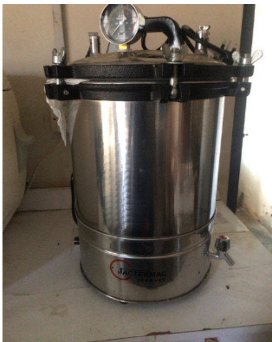
17GH, #046. Benchmark compliant pressure-cooker autoclave, purchased new.
