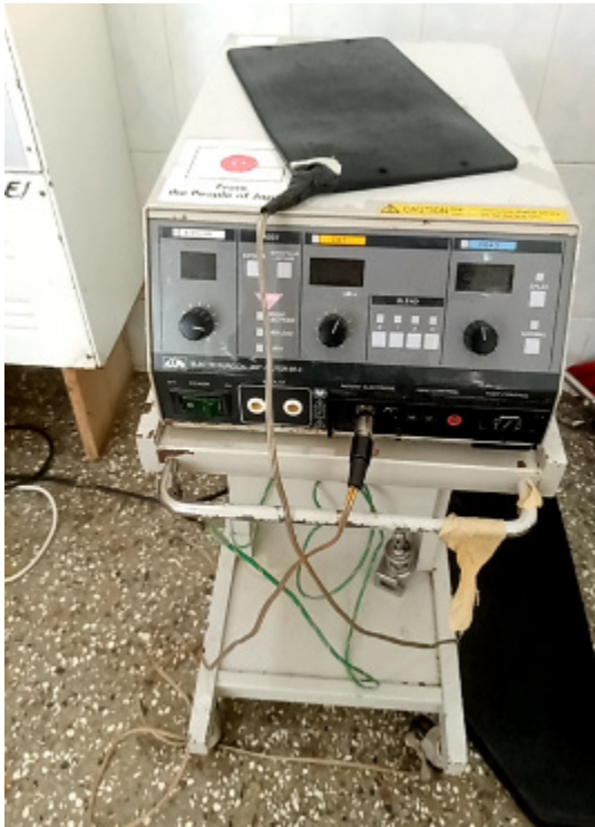
08GH, #002 Used within 7 days but has safety concerns and a faulty grounding plate.
