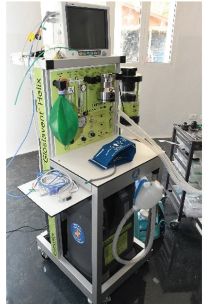
Figure 21. An open circuit anaesthetic machine designed for the LMIC environment.
