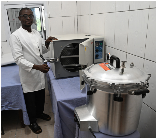
A small hospital in Cameroon with its primary autoclave, together with a secondary autoclave as a backup.
